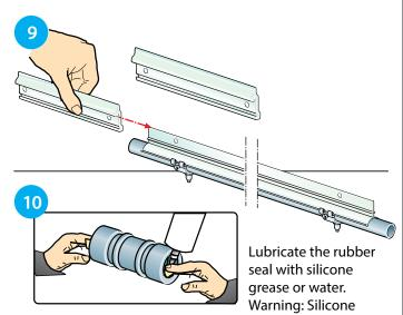
lubricants may be used, but do not use oil, grease or soap as a lubricant: they will damage the components.
